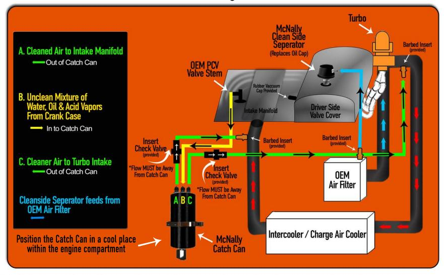
**NOTICE** - We have provided 6 (six) possible installation diagrams for different engine configurations. Please select the correct installation guide. **Before you start KNOW THIS:** The installation of this product in your vehicle requires substantial knowledge of your vehicle's engine and its internal functions. Many "do-it-yourselfers" are fully capable of properly installing this product while others are NOT.
