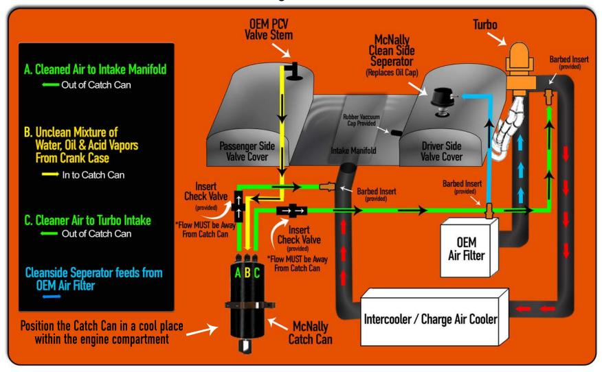
**NOTICE** - We have provided 6 (six) possible installation diagrams for different engine configurations. Please select the correct installation guide. **Before you start KNOW THIS:** The installation of this product in your vehicle requires substantial knowledge of your vehicle's engine and its internal functions. Many "do-it-yourselfers" are fully capable of property installing this product while others are NOT.
